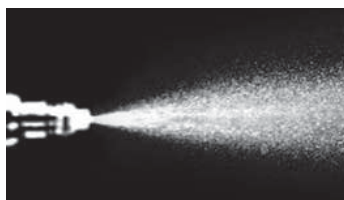
Injector spray pattern after P.i. treatment.
